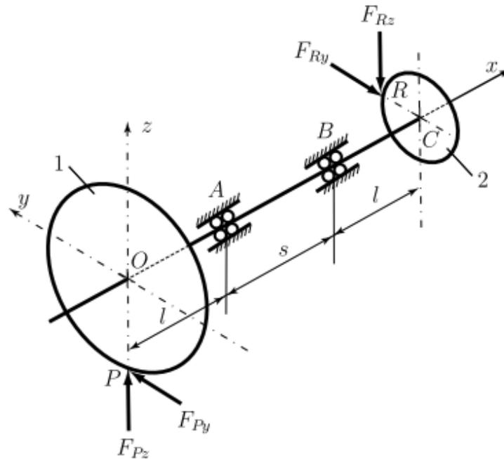
Figure 4. Force diagrams acting on the bearing
