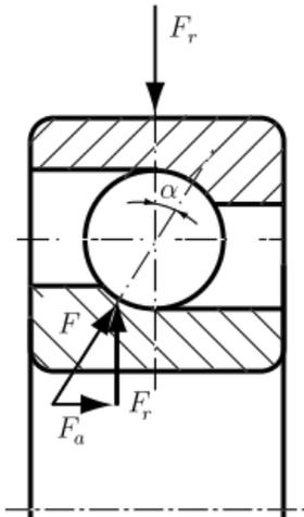
Figure 1. Radial thrust (angular contact) ball bearing
