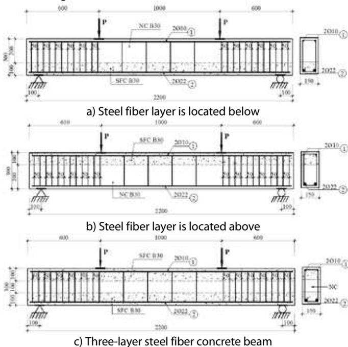
**Fig. 1** Model of two-layer and three-layer concrete beams
