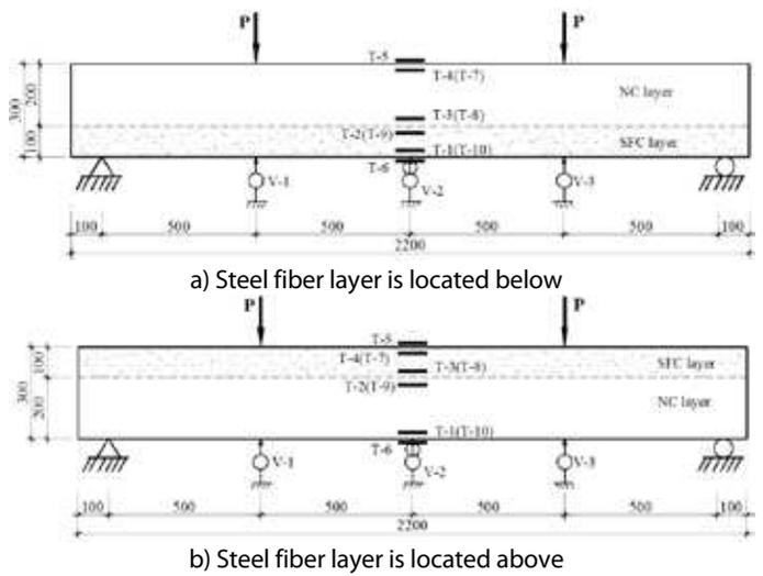
**Fig. 2** Diagram for placing strain and vertical displacement measuring devices in beams
