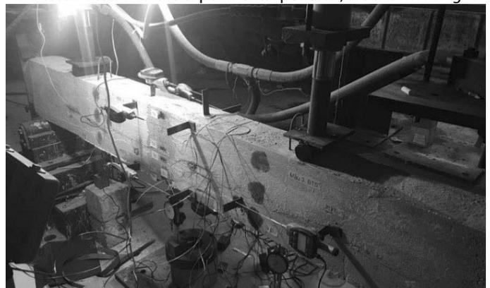
**Fig. 4** Tested beams on the experimental pedestal
