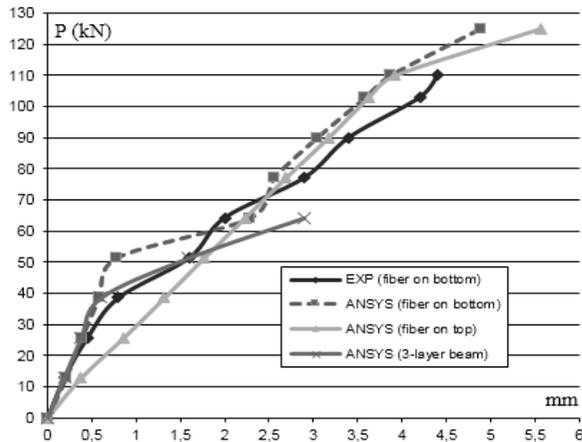
**Fig. 10** Vertical displacement at the middle of the beam span
